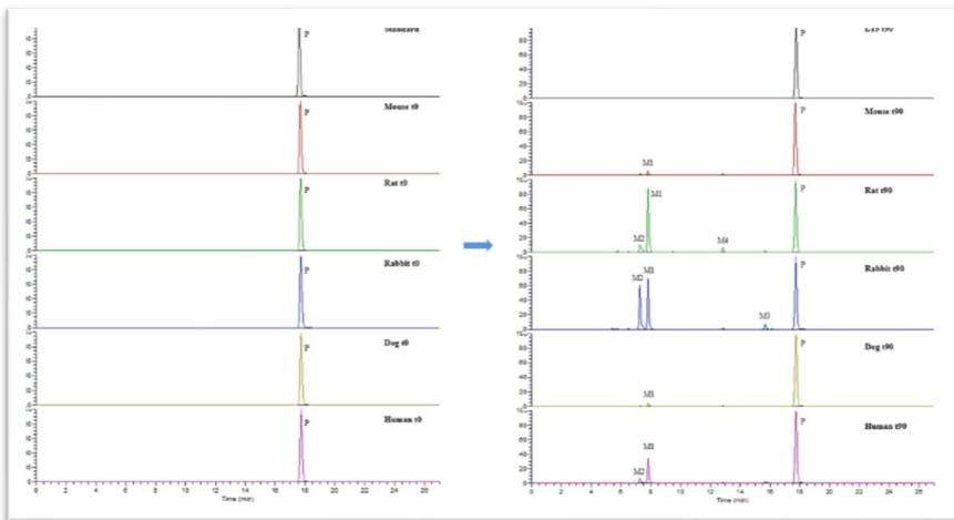
Extracted ion chromatograms at the main metabolites masses in mouse, rat, rabbit, dog and human hepatocytes samples at the start of the incubation (t0) and after 90 minutes incubation at the concentration of 10  $\mu$ M.
