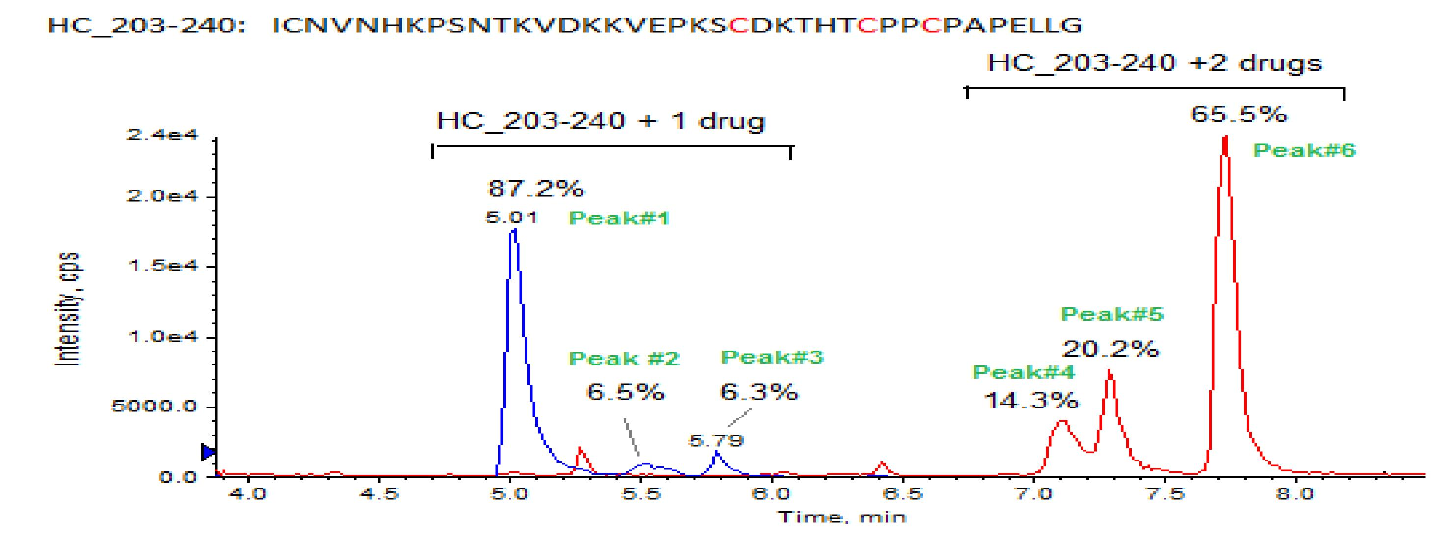
Figure 2. Heavy chain positional isomers separation
