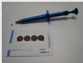
Figure 2. DBS on FTA DMPK Card and 3 mm Micro-Punch
